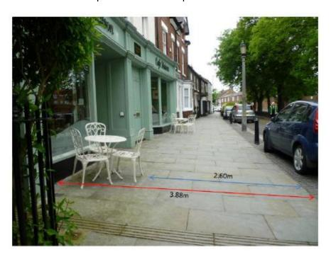
Stockton – Footway width is insufficient to provide adequate a pedestrian clearway of 2 metres
